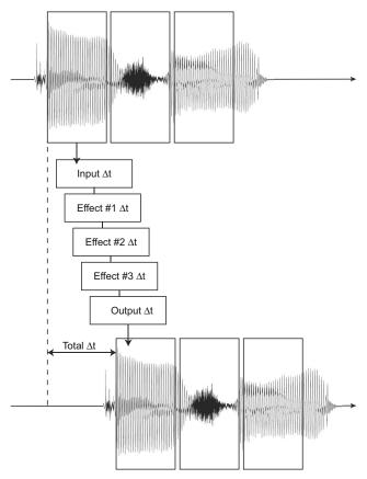
**Fig. 2** Illustration of the delays involved in the realization of our real-time audio processing system. Beyond a baseline I/O latency (input and output  $\Delta_I$ ), each atomic effect in the signal data flow (3 as illustrated here) imparts further delay, which depends on the effect's algorithmic complexity
