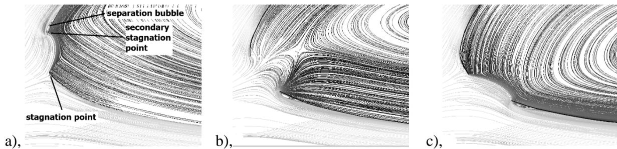
**Figure 10** Streamlines at  $\alpha = 4^\circ$  for  $Sc = 5.3\%$ ,  $Sw = 4\%$
