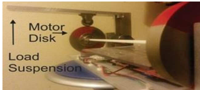
Fig. 7.7 Fabricated mechanical lever type arrangement for load (mass) suspension
