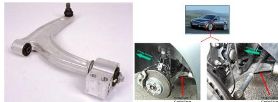
Figure 4: The front lower control arm
