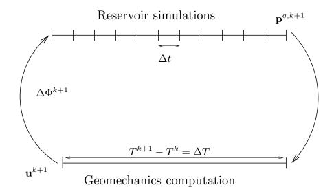
FIGURE 4. Sketch of the iterations between reservoir and mechanical computations on the time period  $\Delta T$ . **5.1. The case of the linear model.** We solve the set of equations (16-17), where  $c_r$  is a relaxation parameter, by means of a fixed point method. The corresponding algorithm, where the iteration parameter is denoted by l, is given by (22)
