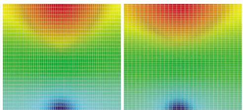
FIGURE 18. Pressure at time t = 100 s where R = 100 and two different meshes: on the left-hand-side with vertically stretched cells and on the right-hand-side with horisontally stretched cells ones.
