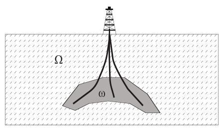
FIGURE 1. The reservoir and the geomechanical domains.
