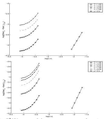
FIGURE 6.  $L^2(\Omega)$ -norm of the error  $\mathbf{u} - \mathbf{u}_h$  as a function of  $\Delta x$ , on the left-hand-side with the staggered algorithm and on the right-hand-side with the preconditioned conjugate gradient algorithm with q = 1,  $c_o = 1$  and  $\Delta t = 0.01$ .
