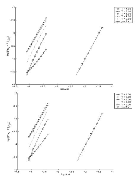
FIGURE 5.  $L^2(\omega)$ -norm of the error  $p - p_h$  as a function of  $\Delta x$ , on the left-hand-side with the staggered algorithm and on the righthand-side with the preconditioned conjugate gradient algorithm with q = 1,  $c_o = 1$  and  $\Delta t = 0.01$ .
