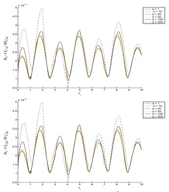
FIGURE 7. The relative error  $p - p_h$  in  $L^2(\omega)$ -norm as a function of time, on the left-hand-side with the staggered algorithm and on the right-hand-side with the preconditioned conjugate gradient algorithm for different values of q with  $c_o = 1$ ,  $\Delta t = 0.01$  and  $\Delta x = 1/40$ .
