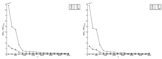
FIGURE 11. The time evolution of the  $(L^2(\Omega))^2$ -norm of the error between the reference solution and the approximate displacements computed for different values of q on the left-hand-side by the staggered algorithm and on the right-hand-side by the preconditioned conjugate gradient algorithm.
