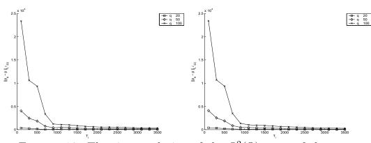
FIGURE 10. The time evolution of the  $L^2(\Omega)$ -norm of the error between the reference solution and the approximate pressures computed for different values of q on the left-hand-side by the staggered algorithm and on the right-hand-side by the preconditioned conjugate gradient algorithm.
