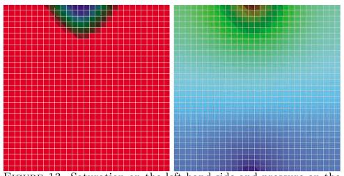
FIGURE 13. Saturation on the left-hand-side and pressure on the right-hand-side at the time t = 100 s with R = 1 on a regular mesh.
