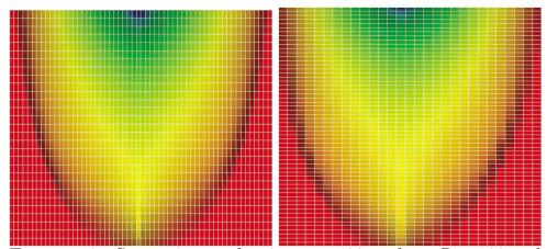
FIGURE 17. Saturation at the time t = 580 s where R = 100 and two different meshes: on the left-hand-side with vertically stretched cells and on the right-hand-side with horisontally stretched cells ones.
