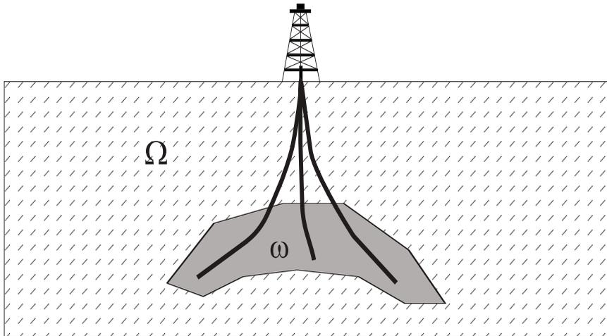
FIGURE 1. The reservoir and the geomechanical domains.
