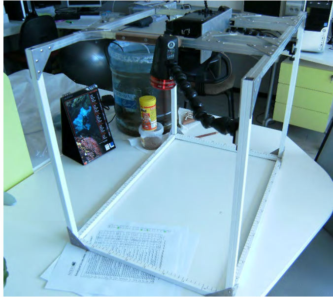
Figure 28. Photoquadrat equipped with a digital camera and 4 SOLA Lights.
