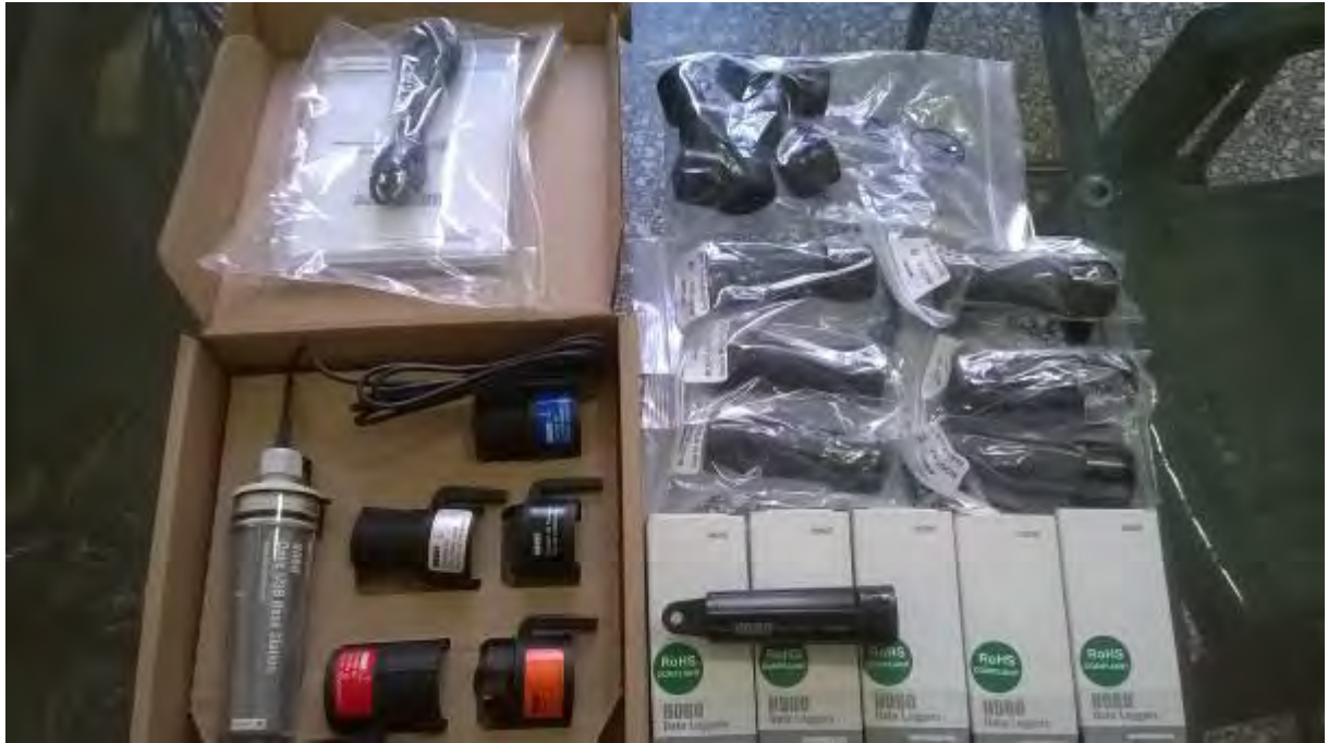
Figure 2: Onset's Waterproof Data Logger system which will be installed at Zakynthos sampling sites for a long-term temperature monitoring.
