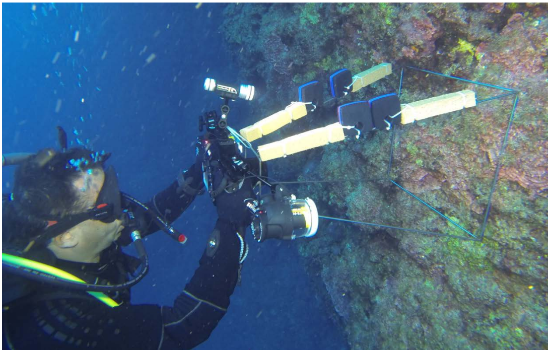
Figure 12. Taking a picture by the photo-quadrate system used in the Turkish stations.
