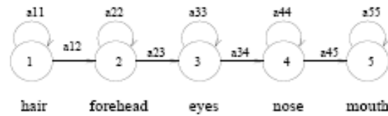
Figure 2: Left to right HMM for face recognition [5].
