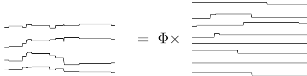
Figure 4: Example of synthesized signal Y = \Phi X , with C = 4 channels and N_{\Phi} = 8 atoms.
