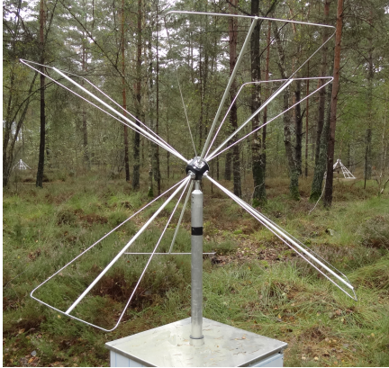
Figure 3. The tripole antenna.
