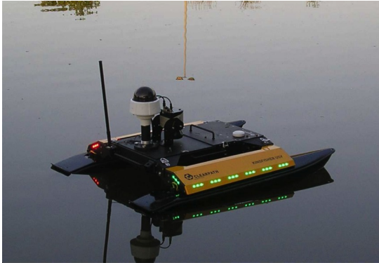
Fig. 2. The Kingfisher on a very smooth lake. The pan-tilt camera is housed in the white dome at the back of the boat, just behind the laser scanner used for navigation.
