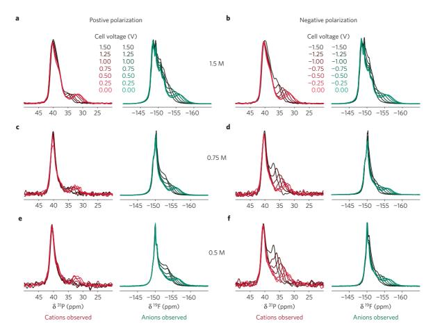
Figure 3 | In situ  $^{31}$ P and  $^{19}$ F NMR spectra of individual supercapacitor electrodes at different states of charge. a-f, Spectra recorded in the range 0 to 1.5 V (a,c,e) and in the range 0 to -1.5 V (b,d,f). Electrolyte concentrations are 1.5 M (a,b), 0.75 M (c,d) and 0.5 M (e,f). In-pore anion intensities increase for positive charging, whereas in-pore cation intensities increase for negative charging.
