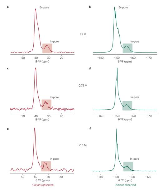
**Figure 1 | NMR** spectra of individual supercapacitor electrodes showing in- and ex-pore cation and anion environments. **a-f**, <sup>31</sup>P (**a,c,e**) and <sup>19</sup>F (**b,d,f**) NMR spectra were recorded for electrolyte concentrations of 1.5 M (**a,b**), 0.75 M (**c,d**) and 0.5 M (**e,f**). Supercapacitors were held at a cell voltage of 0 V. The in-pore resonances in each spectrum are highlighted.
