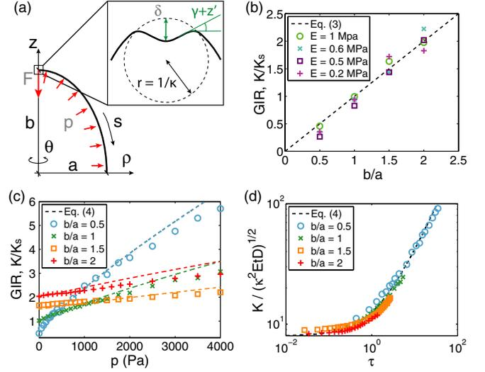
FIG. 2 (color online). Indentation at the pole. (a) Schematic of a deformed ellipsoidal specimen. (b) Dependence of GIR  $K/K_s$  on  $b/a$  for four different elastic polymers and  $p = 0$ . (c) GIR  $K/K_s$ , as a function of the internal pressure  $p$  for four aspect ratios  $b/a = \{0.5, 1, 1.5, 2\}$  and  $E = 1$  MPa. (d) Dimensionless experimental rigidity  $K D / (K_s^2 E I D)$  against dimensionless pressure  $\tau$ .
