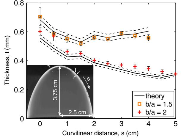
FIG. 4 (color online). Comparison between measured and predicted thickness profile for two unpressurized shells with  $b/a = 1.5$  and  $2$  and  $0.9 < E < 1$  MPa. Solid and dashed lines represent mean value  $\pm$  standard deviation for the predicted thickness. (Inset) Scanned image of a shell with aspect ratio  $b/a = 1.5$  cut in half.
