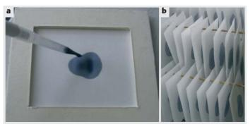
Preparation of test samples: application of a 0.1 mL drop of ink **(a),** samples hanging during drying **(b).**
