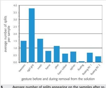
Average number of splits appearing on the samples after removal from the bath. The tested actions are depicted in Tab 1.
