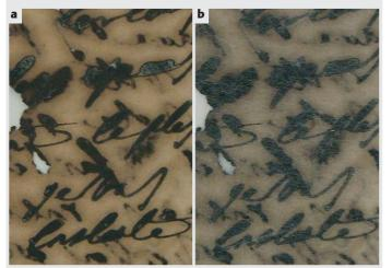
10 Daylight picture of the same document as in Fig 8 (detail): before treatment (a), after treatment (b).
