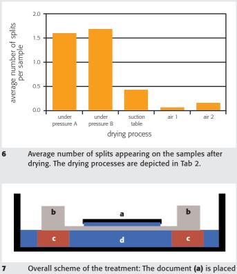
on a silkscreen (b) supported by four blocks (c) at the corners. The tray is filled until the solution (d) reaches the screen. The weight of the document enables water to permeate through the mesh underneath the document only.
