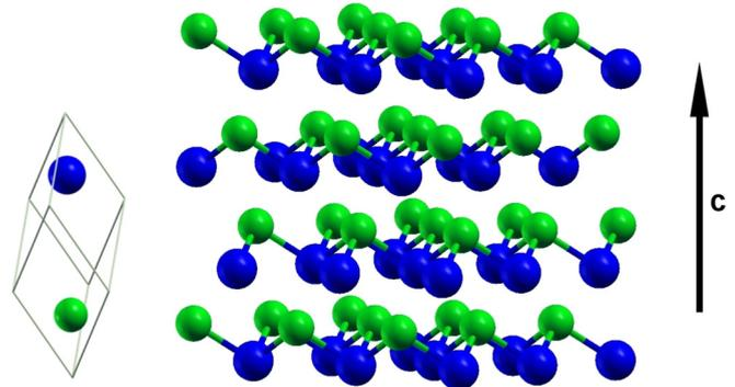
FIG. 1. Geometry of the GeTe crystal seen as a stacking of bilayers along the  $c$  axis of the conventional hexagonal unit cell with the three short intrabilayers bonds and three long interbilayers bonds. Green spheres denote Ge atoms and blue spheres denote Te atoms.
