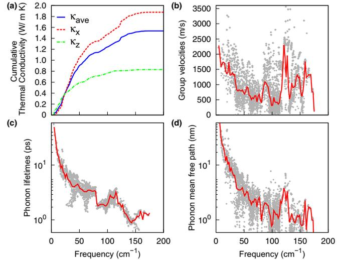
FIG. 10. (a) Cumulative lattice thermal conductivities within the SMA (see text) along the  $c$  axis in the hexagonal notation ( $\kappa_z$ , see Fig. 8) in the perpendicular plane ( $\kappa_x$ ) and their average for a polycrystalline sample ( $\kappa_{\text{av}}$ , see text), (b) group velocities, (c) phonon lifetimes, and (d) mean free paths averaged over a small window of  $2 \text{ cm}^{-1}$  as a function of phonon frequencies in  $\text{Sb}_2\text{Te}_3$  crystal at 300 K.
