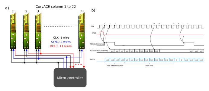
The main supply voltage was decoupled and divided into one for the analogue circuitry and another for the digital circuitry (four pads). The further processing of the photodiode output signals via a multiplexer (MUX) and the ADC is shown in Figure 4 (three pads for sync, clock and data lines). The remaining pad
