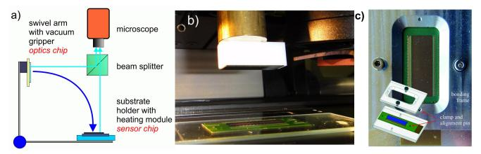
In contrast, the mounting of this stack onto the flexible PCB was done passively with a jig aid by means of two-component epoxy glue (EPO-TEK 353ND). Therefore, an adapted assembly stage was used, which allowed for a fast bonding process at an adequate lower level of precision due to a mechanical guide pin (see Figure 9c).
