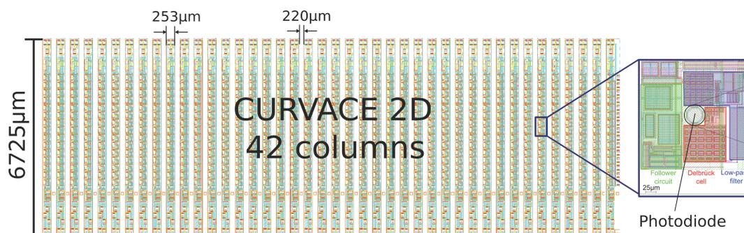
In general, the layout is the same for all columns, except the most right one, which possesses additional readout test pads for each photodetector. As shown in Figure 2 and in the Figure S2 of the Supplementary Data published in [2], a column consists of 15 photodetectors followed by Delbrück circuits [27], a 16-channel multiplexer (MUX), a 10-bit analog-to-digital converter (ADC), a state-machine and eight electro-static discharge (ESD) shielded pads for wire bonding. An additional
