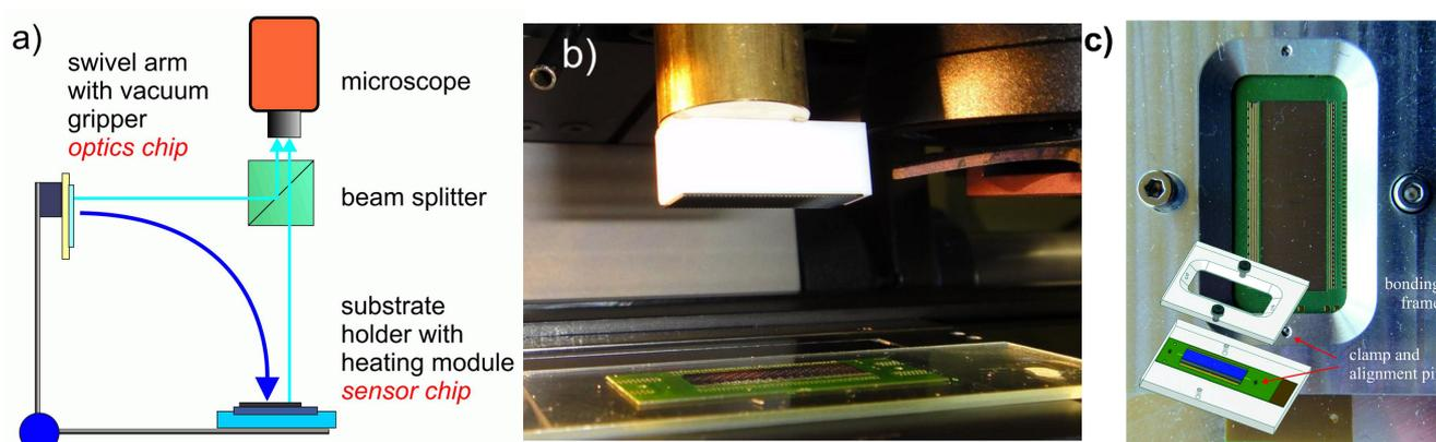
In contrast, the mounting of this stack onto the flexible PCB was done passively with a jig aid by means of two-component epoxy glue (EPO-TEK 353ND). Therefore, an adapted assembly stage was used, which allowed for a fast bonding process at an adequate lower level of precision due to a mechanical guide pin (see Figure 9c).
