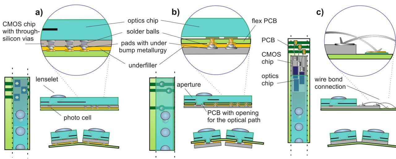
In the first step, the required components have been prepared for stack mounting. The VLSI and the microoptics chips have been diced from eight-inch and four-inch wafers, respectively. Moreover, the sensor chips have trenching grooves at their backside at the positions of the dicing lanes. These trenches of  $100\ \mu\text{m}$  in depth and  $150\ \mu\text{m}$  in width allowed for safe cutting at a later step.
