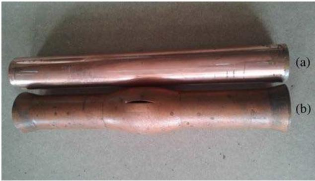
**Fig. 7** **a** Non-annealed copper tube and **b** annealed copper tube (exploded)
