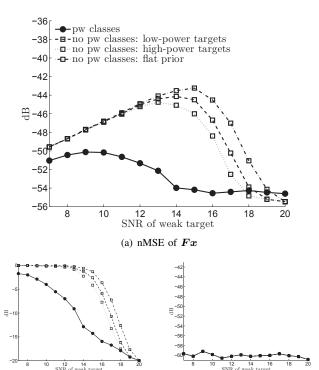
Fig. 3. Comparison between the performance of the proposed algorithm with power classes (plain line), and that of the previous algorithm from [6] in the case of a flat prior (dash-dotted line), or a prior adjusted to high-power (dotted line) or low-power targets (dashed line). The scenario consists of three close targets separated by 1/M.  $\bar{M}=M=16$ .  $N_r=1000$ ,  $N_{bi}=200$ .
