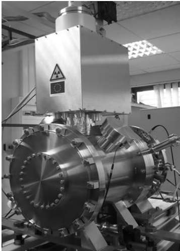
Figure 1. Irradiation chamber MATSPACE equipped with a 100 keV electron gun.
