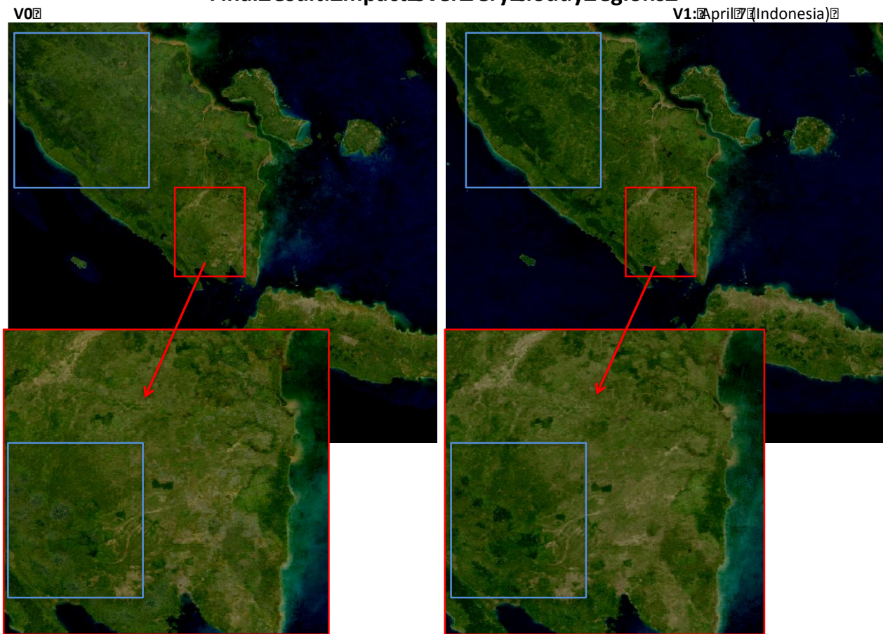
Fig. 6 Impact of the reconstruction in a very cloudy region of Indonesia; it illustrates that the canopy is less noisy in V1 (right) than in V0 (left).
