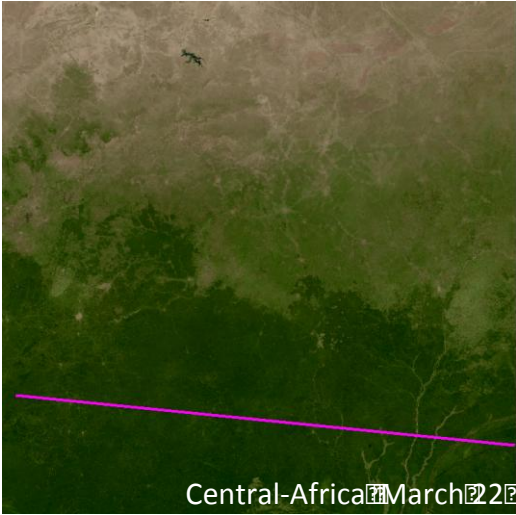
Fig. 8 Impact of our reconstruction method over deep forest. The right hand side graphs display the reflectance values computed across the magenta transect for the red, green and blue visible bands, as computed by V1 (colored lines) and V0 (black lines), highlighting the improvements brought by the V1 FondsDeSol algorithm. The quoted V1/V0 values are the ratios between the mean values of the two FDS versions. The horizontal lines represent the mean values of each data sets.
