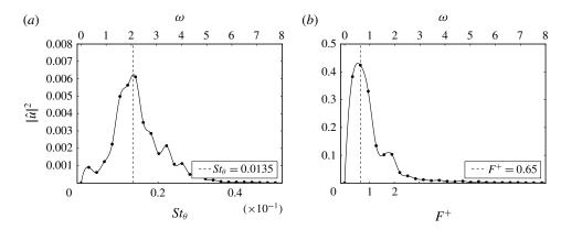
FIGURE 2. Spectra of the streamwise (spanwise-averaged) velocity computed from the unsteady ZDES simulation at two locations: (a) x = 2, y = 1.5, (b) x = 7.0, y = 0.1.  $St_{\theta}$  is the Strouhal number based on the free-stream velocity and the momentum thickness at the step location, and  $F^+$  the Strouhal number based on the free-stream velocity and the reattachment length.
