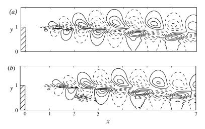
FIGURE 7. Comparison between the real part of the streamwise velocity of (a) the dominant optimal response and (b) the PSE field, for  $\omega = 2.1$  (normalised in phase and amplitude). Each figure displays ten equally spaced contours ranging from -1 to 1.
