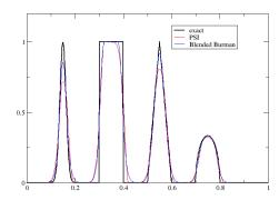
Figure 2: Results for the convection problem with initial conditions (46), at T=8 with quadratic elements. The results are obtained with  $B\ell$ -PSI<sub>3</sub> (quadratic elements). Only 3 iterations are made. The mesh has 400 cells (3 degrees of freedom per element).
