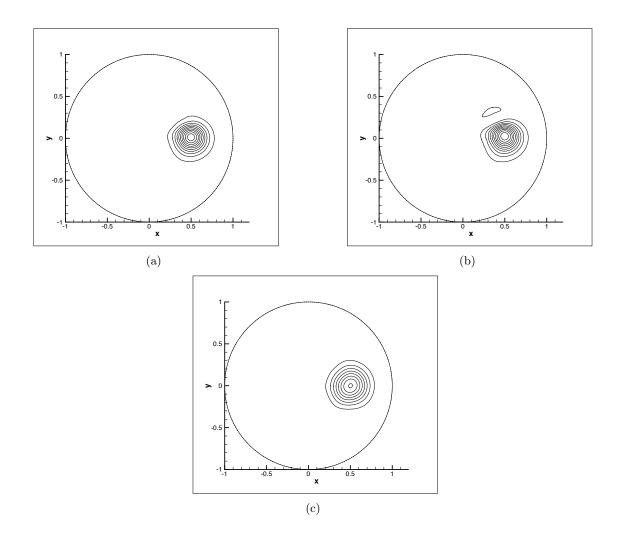
Figure 4: Results for the  $\mathbb{P}^1$  approximation: (a) with SUPG, after 1 rotation, (b) with SUPG after 2 rotations, (c) with Burman residual after 10 rotations. The same isolines are represented.
