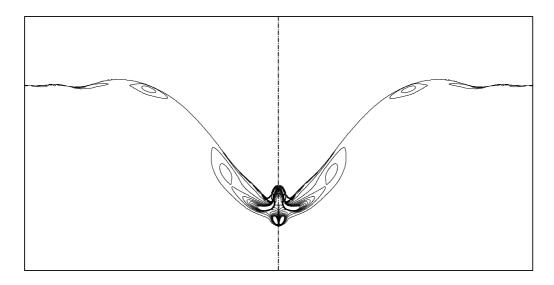
Figure 4: Vorticity isolines during the collapse of the bubble for the same conditions as in Fig. 3.
