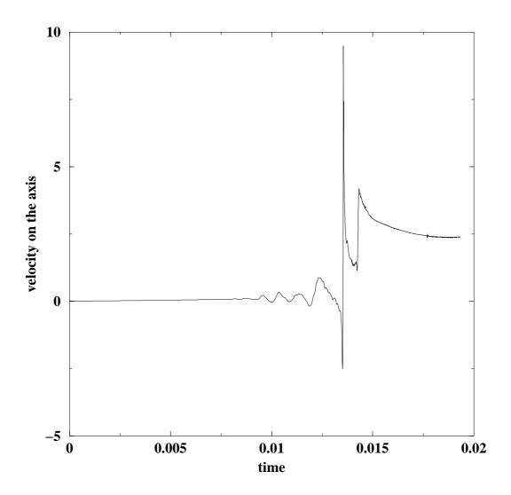
Figure 11: The velocity of the interface on the axis for  $R/R_{\nu} = 2.88 \, 10^5$ . The oscillations correspond to the arrival of a train of capillary waves. For this large value of  $R/R_{\nu}$  capillary waves are numerous and of short wavelength. The very large excursion in velocity may be due to the existence of a further bubble entrapment region, however the very small scales involved make numerical resolution difficult.
