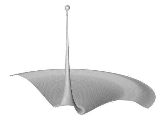
Figure 1: Jet produced by the collapse of a spherical cavity. The end droplet will eventually detach due to the Savart-Plateau-Rayleigh instability.
