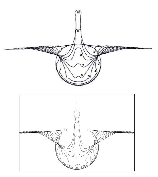
Figure 3: Time sequence of the jet formation in a  $2.57\mu l$  bubble bursting at a free surface. Top: experimental [7] and bottom: computational results. Profiles are 1/6000s. apart.
