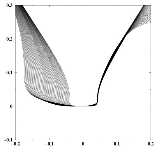
Figure 15: Comparison between successive profiles made non-dimensional using the scaling  $\eta = x/(t_0 - t)^{2/3}$  described in the text. Left: unrescaled profiles. Right: rescaled profiles. There the opening angle of the cavity is around 73°. Since the numerical method uses adaptive time-stepping, the profiles are not separated by equal time intervals.
