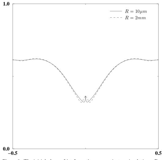
Figure 9: The initial phase of jet formation as seen in two simulations. For the large bubble (dashed line,  $R/R_{\nu} = 14400$ ) the jet is relatively wide and well resolved numerically. For smaller bubbles (solid line,  $R/R_{\nu} = 720$ ) the jet may become extremely thin.
