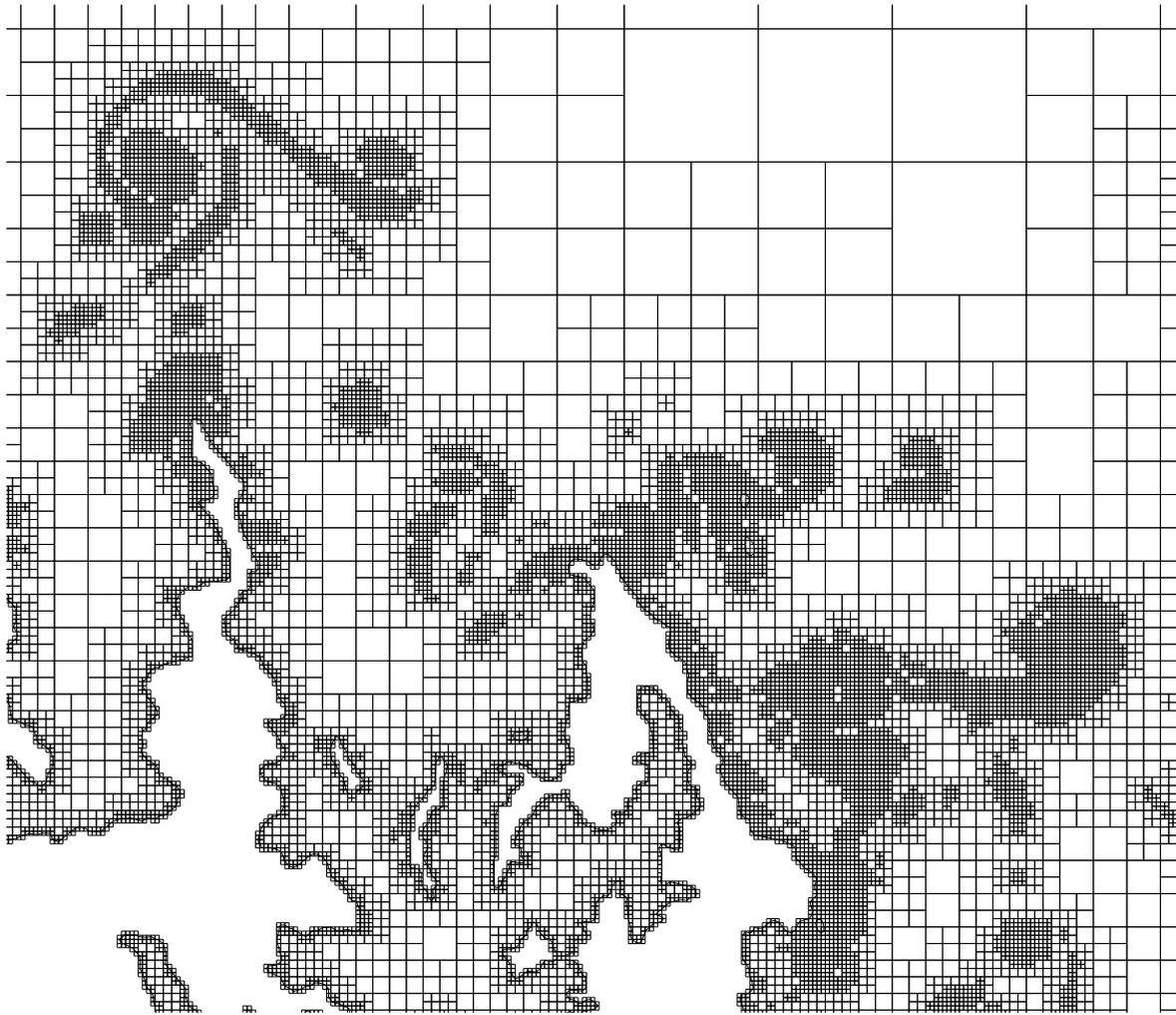
Figure 12: Detail of the adaptive quadtree mesh. The coastline is statically refined at the finest level while individual eddies are tracked dynamically. The domain extent is  $36 \times 29$  km. The minimum spatial resolution is 122 metres.
