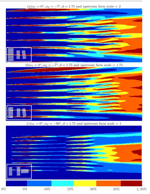
$\textbf{Fig. 11} \ \ \text{Mean flow reduction in percent.} \ \ \text{The mean flow reduction in the wake of the farm blocks is mainly dependant of the aspect ratio of the farm blocks.}$
