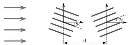
Fig. 6 The first set of simulations was realized using 2 farm blocks of 5 long-lines in a laminar flow. The 3 parameters of the simulation are the distance between both farm blocks, d, and the angle between each farm block and the inflow direction,  $\alpha_1$  and  $\alpha_2$ .
