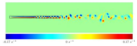
Fig. 5 Flow past a single long-line parallel to the mean flow direction. The shear caused by the long-line induces vortex shedding in the wake of the long-line. Vortices are forming within the long-line and then expelled in the wake.
