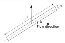
${\bf Fig.~4} \ \ {\bf Schematic \ representation \ of \ a \ long-line \ as \ used \ in \ the \ simple \ analytical \ model}.$
