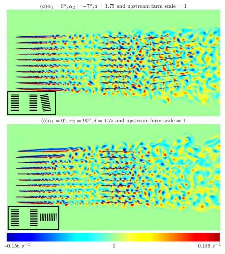
Fig. 10 Vorticity field for a turbulent flow past two farm blocks at angles  $(\alpha_1, \alpha_2) = (0, 7)$  (top) and (0, 90) (bottom). The importance of the angle between flow direction and farm is neat with the long-lines being regions of high vorticity for small angle (top) and almost no interaction noticeable for large angles (farm 2 - bottom).
