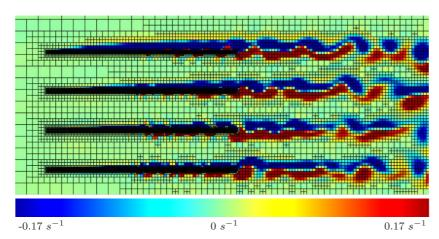
${f Fig.~3}$  Adaptive mesh near long-lines. Fine resolution of the long-lines allows accurate representation of the long-line area where the drag term corresponding to the mussel 'droppers' is applied. Vortical structures generated by the long-lines are "followed" by the adaptive grid.
