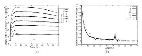
Fig. 14 Results from the "simple model". (a) Integral of the reduction in velocity over the wake behind a farm block versus farm block angle for blocks made of 4 to 16 long lines. (b) Difference between the local maximum and minimum reduction in flow in the wake behind a farm block versus farm block angle for blocks made of 4 to 16 long lines. The triangular points labelled "model" correspond to the simulation made using the Gerris Flow Solver. The peak at  $52 \circ$  is a numerical artefact.
