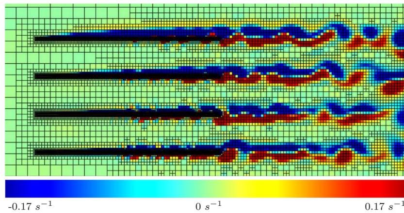
**Fig. 3** Adaptive mesh near long-lines. Fine resolution of the long-line area allows accurate representation of the long-line area where the drag term corresponding to the mussel 'droppers' is applied. Vortical structures generated by the long-lines are "followed" by the adaptive grid.
