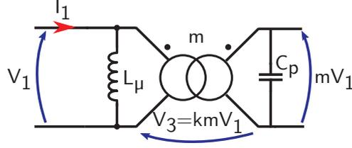
Fig. 6: Low frequency electrical model of a two winding transformer when  $V_3$  is known as a function of  $V_1$ .
