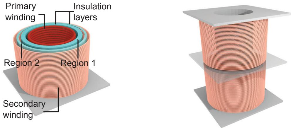
Fig. 3: Construction of a two sections / two layers ( $N_s = 2 / N_l = 2$ ) transformer. Magnetic core not presented.
