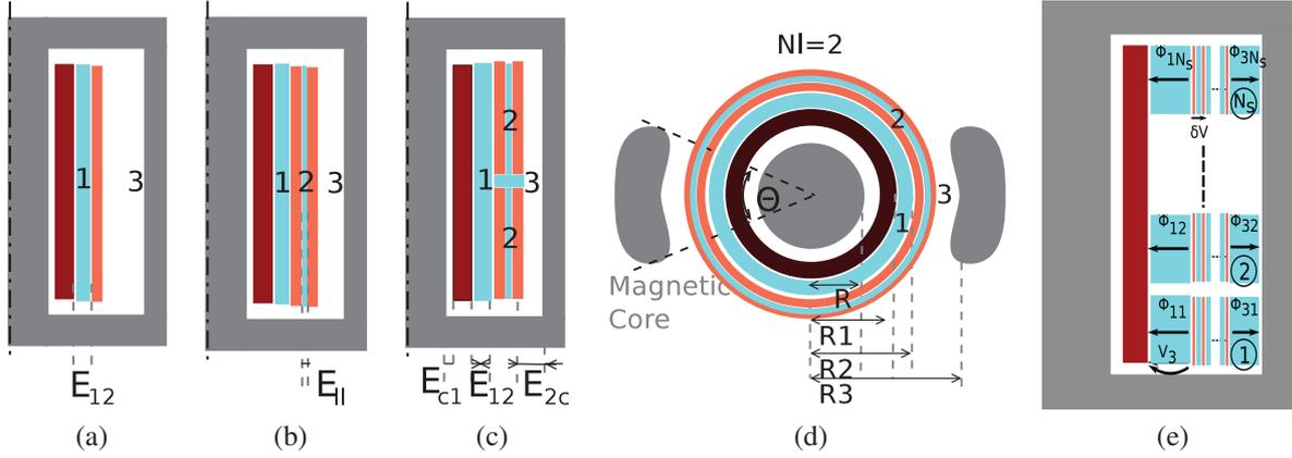
Fig. 4: Internal structure of the three transformers under study.  $N_l = 1$  in (a),  $N_l = 2$  in (b) and (c);  $N_s = 1$  in (a)(b) and  $N_s = 2$  in (c).  $N_l$  and  $N_s$  are respectively the numbers of layers and sections in the secondary winding. General case (e).
