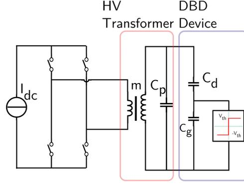
Fig. 1: Current controlled source to supply DBD devices
