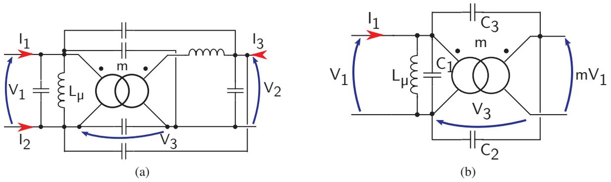
Fig. 2: Lossless transformer model. General model (a) and low frequency model (b).
