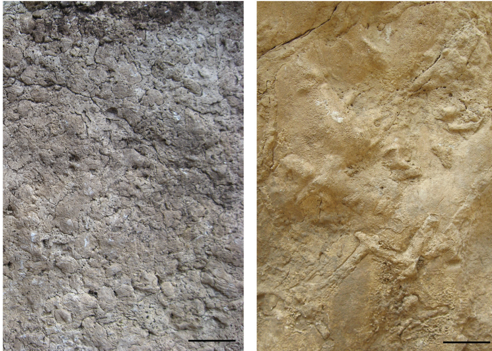
Fig. 8 – Fontenille, Motte de la Jacquille (Charente, France): macroscopic aspect of the facies used for the orthostats in the funerary chamber (scale: 5 cm); left: conglomeratic gravelly; right: grainy limestone with fucoids (photos D. Poncet).
