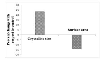
Fig. 2. Percent change in crystallite size and surface area of treated sample of p-chlorobenzonitrile as compared to control.
