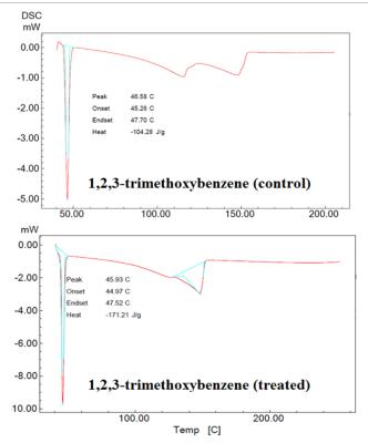
Figure 3: DSC thermograms of control and treated 1,2,3-trimethoxybenzene.
