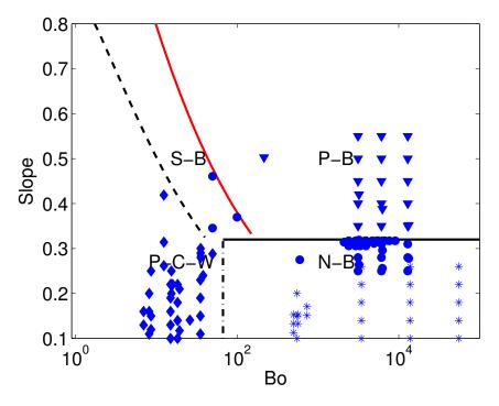
Figure 11: Wave state diagram, compares the regimes obtained through the simulation and described in fig. 7 with the experimental studies summarized in table 1. Experimental studies: \*: breakers triggered by modulation instability,  $(\mathbf{\nabla})$ : plunging breakers,  $(\bullet)$ : spilling breakers,  $(\mathbf{\Phi})$ : parasitic capillary waves
