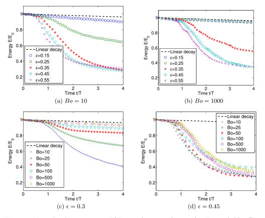
Figure 9: Normalized wave energy  $E/E_0$  as a function of time t/T. Figure (a,b): effect of increasing steepness for (a) Bo = 10 and (b) Bo = 1000. From top to bottom  $\epsilon =$ 0.15, 0.25, 0.35, 0.45 and 0.55. Figure (c,d): effect of increasing surface tension at a given steepness, (c)  $\epsilon = 0.3$  and (d)  $\epsilon = 0.45$ . From bottom to top Bo = 2, 5, 10, 20 and 100. Black dashed line is the theoretical linear viscous dissipation  $E/E_0 = \exp(-4\nu k^2 t)$ .
