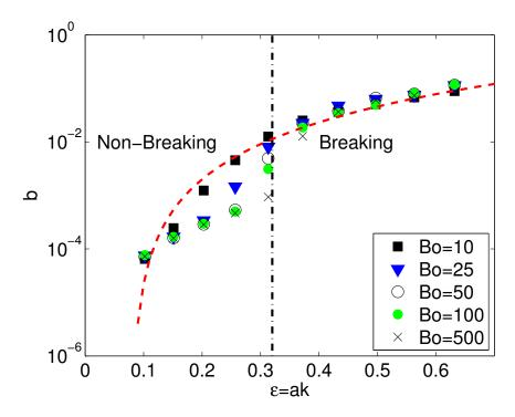
Figure 10: Breaking parameter b as a function of steepness for various Bond numbers. Red dashed line is the semi-empirical dissipation function:  $b = 0.4(\epsilon - 0.08)^{5/2}$  (eq. 4.6) from Romero *et al.* (2012). Vertical dot-dash line indicates the breaking threshold in the present work,  $\epsilon_c = 0.32$ .
