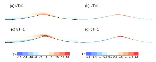
Figure 1: Non-breaking gravity waves propagating to the right and the vorticity field  $\Gamma^* = \Gamma/\Gamma_0$  at t/T=1, for two different steepness: 0.2 (a,b) and 0.25 (c,d). The vorticity field is displayed both in the air and water (left) and only in the water (right) with different color-scale.  $Re = 4 \times 10^4$ , Bo = 1000. We can see that the wave is more asymmetric for  $\epsilon$ =0.25, due to stronger non-linear effects.
