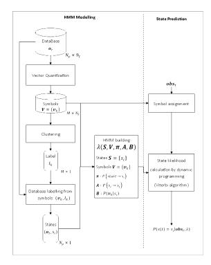
Fig. 2. Hybrid HMM building scheme. Dotted line separates HMM modelling on left side from state prediction of a new observation  $obs_t$  on right side.
