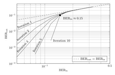
Fig. 8. Output BER as a function of the input BER for the rate 1/2 LDPC code of the DVB-S2 standard over an AWGN channel. In this configuration, the convergence threshold is given at BER<sub>in</sub> = 0.15.
