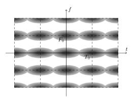
**Fig. 1.** Time–frequency representation of a multicarrier signal. In this example, the generator g(t) and the parameters  $T_0$  and  $F_0$  are chosen in order to show a clear separation in frequency, but not in time.
