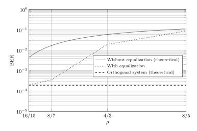
**Fig. 11.** BER as a function of  $\rho$  for a multicarrier FTN system using a DFE,  $E_{\rm b}/N_0=8$  dB and a TFL generator.
