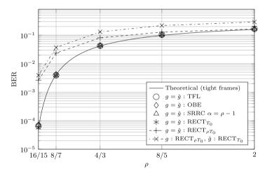
**Fig. 6.** BER versus  $\rho$ , with  $E_{\rm b}/N_0=20$  dB.
