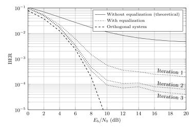
**Fig. 10.** BER as a function of  $E_{\rm b}/N_0$  for a multicarrier FTN system using a DFE, a density  $\rho=8/7$  and a TFL generator.
