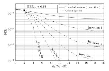
**Fig. 9.** BER as a function of  $E_{\rm b}/N_0$  for a system using the rate 1/2 LDPC code of the DVB-S2 standard (10 iterations of the decoder), a density  $\rho = 4/3$  and a TFL generator. The convergence threshold happens at the value of  $E_{\rm b}/N_0$  corresponding to the expected BER<sub>in</sub> (determined using Fig. 8).
