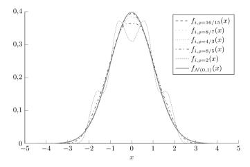
**Fig. 4.** Comparison of the PDF of the interference and its Gaussian approximation with respect to the density ho.
