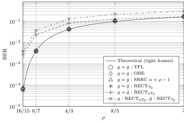
Fig. 6. BER versus  $\rho$ , with  $E_b/N_0 = 20$  dB.
