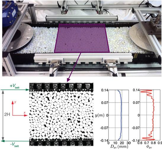
FIG. 1 (color online). Stadium shear device: 2000 plastic cylinders set on a glass plate are sheared by a belt system. Time averaged profiles ( $V^{\text{belt}} = 0.1 \text{ m/s}$ ) of average particle diameter (blue or dark gray) and solid fraction (red or light gray). In the center of the flow,  $D_{\text{av}} \approx 18 \text{ mm}$  and  $\phi_{\text{av}} \approx 0.80$ .
