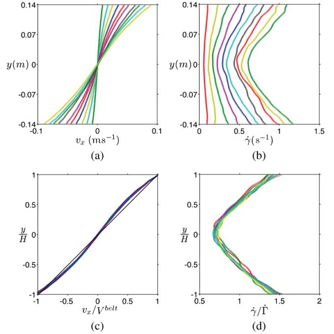
FIG. 2 (color online). (a) Velocity profiles and (b) shear rate profiles for all the runs. The profiles are temporospatial averages of data from the captured central region, which is approximately  $368 \text{ mm}$  wide, over the entire duration of the test. (c) The normalized velocity profiles and (d) the normalized shear rate profiles (where  $\dot{\Gamma} = V^{\text{belt}}/H$ ). In (c) the linear profile (solid black line) has been included for comparison.
