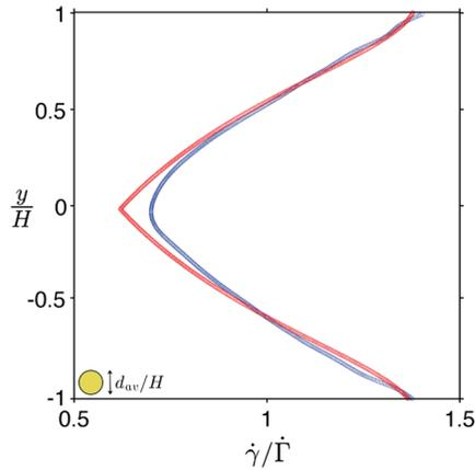
FIG. 4 (color online). The prediction of the model of Eq. (5) with  $a = 0.21$  (red or light gray). The normalized average shear rate profile, i.e., the average of the profiles shown in Fig. 2(d) (blue or dark gray).
