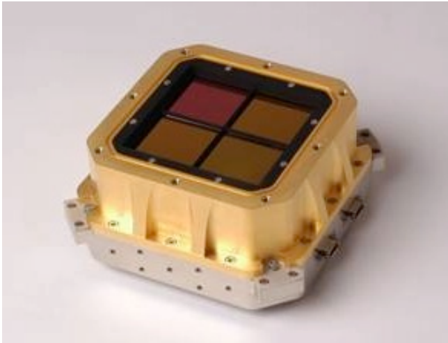
FIG. 1.— Illustration of the 2 \times 2 mosaic CFHT/WIRCam detector array. Each chip features a HAWAII2-RG near-infrared HgCdTe detector with 18 \mu\text{m} pixels. The patrol field has 2040 \times 2040 active pixels with a 4-pixel wide border of reference pixels per chip. The field of view of the full detector array is about 21' \times 21' with 45'' wide inter-chip gaps. Image courtesy of Academia Sinica Institute of Astronomy and Astrophysics (ASIAA).
