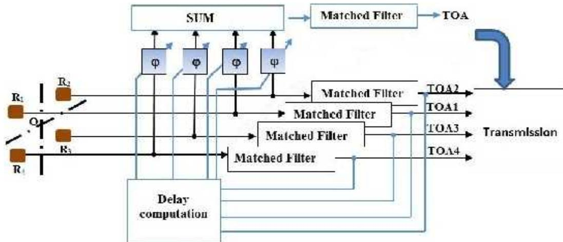
Figure 5. The beamforming algorithm diagram
