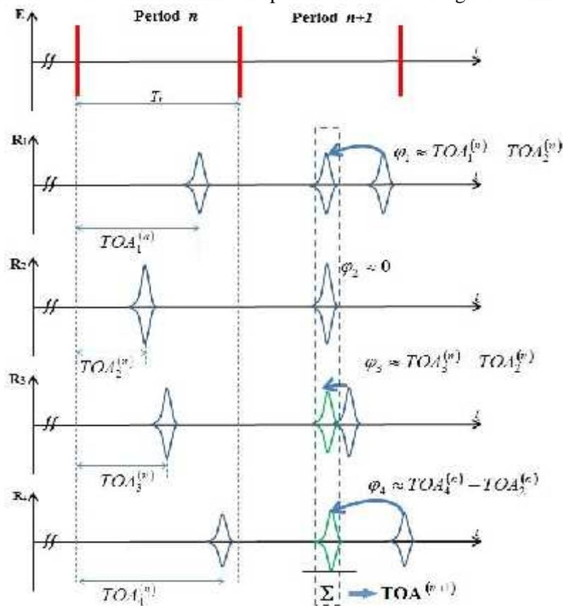
Figure 4. The beamforming algorithm principle
