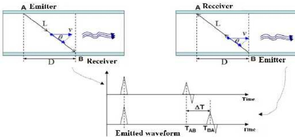
Figure 2. The illustration of the time of flight difference ( $\Delta T$ ) estimation (where  $L$  is the traveled ultrasonic wave physical distance,  $D$  is the distance between the emitter (point A) and the receiver (point B),  $\theta$  is the emission angle and  $T_{AB}$  and  $T_{BA}$  are the time of flight values for the emitted waves in both directions)
