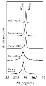
Figure 3: Details of the <111> X-ray diffraction peak shape obtained on: the starting TiC powder; TiC extracted from the Ti matrix after the high-energy ball milling step and TiC extracted from the Ti matrix after 5 min and 450 h of heat treatment at 920°C. The intensity of each diffraction pattern is given in arbitrary units.
