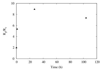
Figure 11: Change in the ratio between the mean size of particles (R<sub>p</sub>) and coherent domains (R<sub>c</sub>) of the TiC powder extracted by acid etching from a Ti-15vol.%TiC compact as a function of heat treatment times at 920°C.
