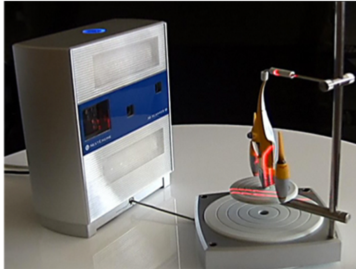
Figure 1. NextEngine 3D Laser Desktop HD
