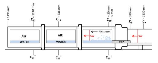
Fig. 1 Scheme of the T200 experimental section and principles of the experiment. The  $C_7$  and  $C_9$  pressure sensors allow for the determination of the Mach number of the incident shock wave. The  $C_{10}$ ,  $C_{15}$ ,
