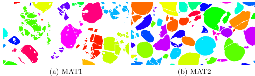
Fig. 7. Results of the fragments merging method.(a) Slice of reassembled MAT1. (b) Slice of reassembled MAT2. In (a), grains are heavily fragmented such as the green grain in the top-right corner, and heavily clustered such as red and yellow grains in the bottom-right corner. In (b), less fragmentation is observed but there is more connections between grains.
