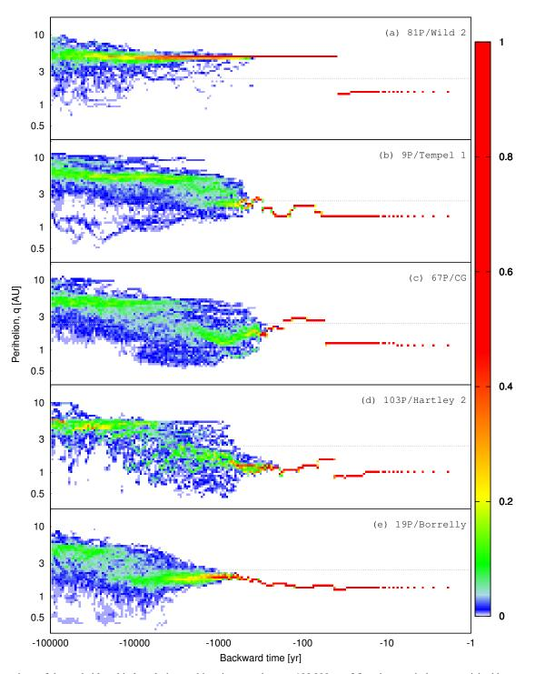
**Fig. 10.** Comparison of the probable orbital evolutionary histories over the past 100 000 yr of five short-period comets visited by spacecraft. The color scale denotes the probability of orbital distribution of a comet in a certain time interval.
