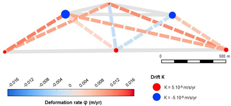
**Figure 2.** Rates of baseline changes obtained from a least squares inversion of baseline and sound speed data, with both constrained sensor drift ( $k$ ) and baseline deformation rate ( $\phi$ ), i.e., assuming no strain on either sides of the fault (paths represented by grey lines). Deforming baselines are shown by dashed lines; colors indicate the magnitude and sign of baseline length variation. Drift in the sound speeds is represented by circles of size proportional to the drift magnitude.
