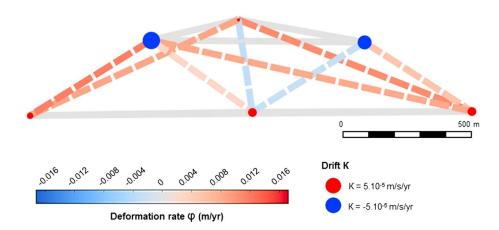
**Figure 2.** Rates of baseline changes obtained from a least squares inversion of baseline and sound speed data, with both constrained sensor drift (*k*) and baseline deformation rate ( $\phi$ ), i.e., assuming no strain on either sides of the fault (paths represented by grey lines). Deforming baselines are shown by dashed lines; colors indicate the magnitude and sign of baseline length variation. Drift in the sound speeds is represented by circles of size proportional to the drift magnitude.
