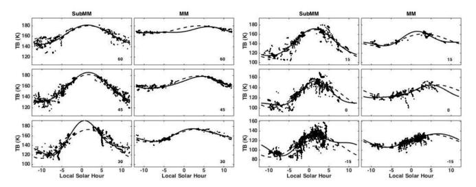
Fig. 2. Data obtained for the SubMM and MM channels in 4 degree wide bins of effective latitude are fit to a Fourier series. The SubMM and MM data for each bin are shown side-by-side; the effective latitude is shown in the lower right of each panel. Models that include both the first and second harmonics in the Fourier Series (solid) and models that only include the first harmonic terms (dashed) have been fit to each set of data.
