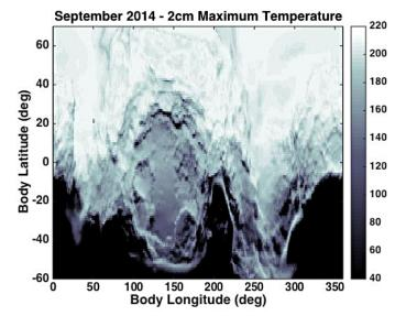
Fig. 11. Maximum temperature at a depth of 2 cm for the I = 22 thermal inertia model, which falls closest to our best fitting values. The thermal model does not include the effects of water ice sublimation and probably over estimates the temperatures in high latitude regions.
