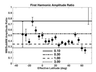
Fig. 6. Ratio of the amplitude of the MM diurnal brightness temperature to the SubMM amplitude. The horizontal lines show expected ratio for different values of  $\delta_{\text{SubMM}}$  under the assumption that  $\delta_{\text{MM}} = 4\delta_{\text{SubMM}}$ .
