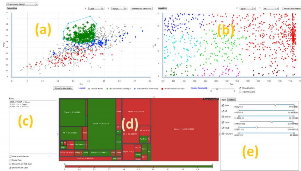
Fig 4. Screenshot of live system: (a) scatter plot of performance output variables; (b) scatter plot of design input variables (showing clustering results); (c) text representation of decision rules; (d) treemap visualization of decision tree; (e) adjustable sliders for ranges of input and output variables (Yan et al. , 2011, 2012)
