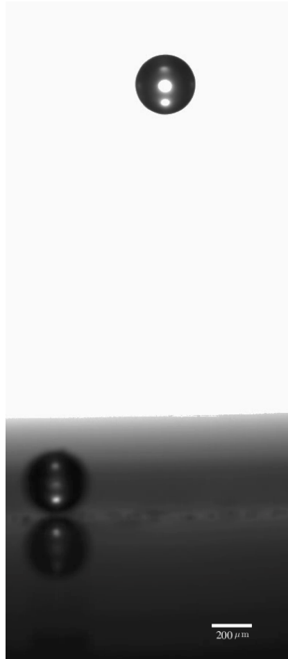
Figure 5: Photograph of a 340\mu\text{m} diameter polystyrene sphere trapped in vertical acoustical tweezers. The trapped particle was selected among others that were lying on a thin polyethylene film. Adapted from [27]
