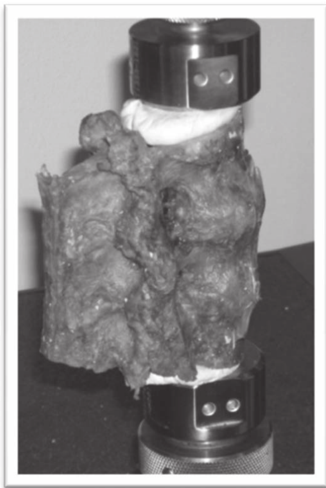
Figure 3. Loading apparatus for mechanical testing of the vertebral motion segment in compression.
